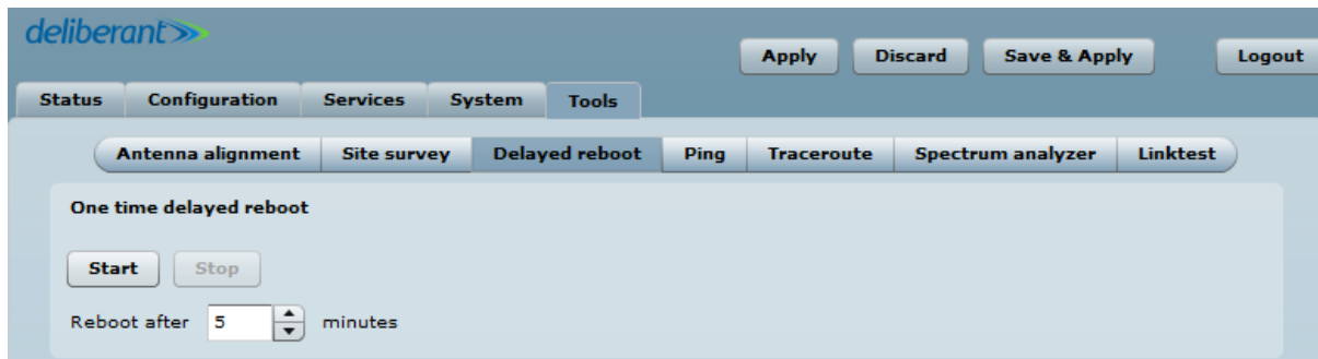
Figure 63 – Delayed Reboot Configuration
